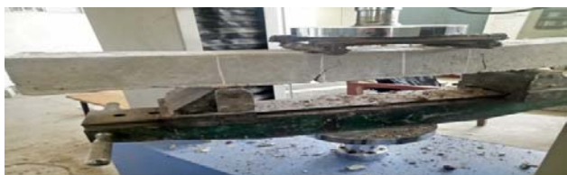
5(e) flexure crack in beam specimen pt: 3.92(a/d=1.25)
