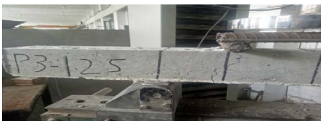
5(d) flexure crack in beam pt: 3.92(a/d=1.25)
